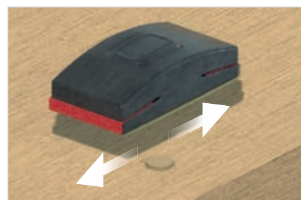
6. Sanding lengthwise (grain #24)
